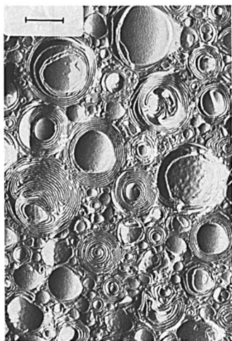
Figure 8. FF-TEM micrograph in the L_\alpha phase with a total surfactant concentration of C_{14} DMAO + C_{14} TAB of 100 mM (ratio of 9:1) with 200 mM hexanol. Bar equals 1 \mu\text{m} .
